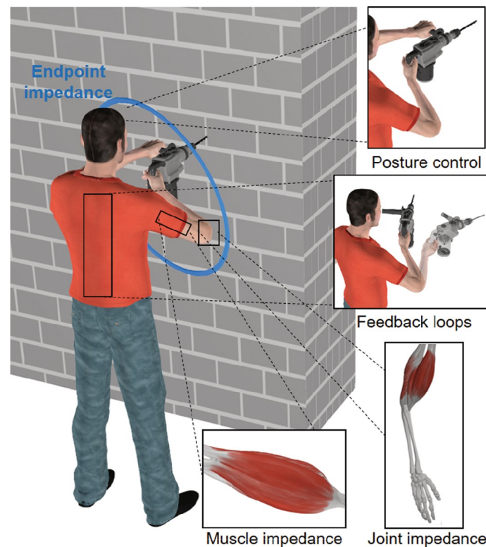
Figure 10 Our ability to stabilize and effectively move our limbs depends, among other factors, on mechanisms at the musculoskeletal level. This is especially evident during the operation of marginally stable objects, which by nature increase the control complexity. For example, when we operate a drill, we apply a large amount of force on the drill pivot point where any small deviations from the vertical axis due to noise can result in loss of stability. While the transformation between the electrical and mechanical signals in the muscle filters some of the noise, to resist any unpredictable perturbations, we increase the impedance of our hands in directions in which it is more likely to experience instabilities (blue ellipse marks the impedance magnitude in different directions). To do so, we can choose a posture for our arms which will generate the greatest increase in impedance once we elevate the cocontraction of muscle pairs. Together, with these noise filtering and stabilization mechanisms, if we unexpectedly lose our original posture, fast feedback loops generate an immediate response, such as the stretch reflex, that resists this sudden change. Such reflexive responses provide the initial solution to losing stability, which will later, due to delay, be complete with additional corrective responses.
