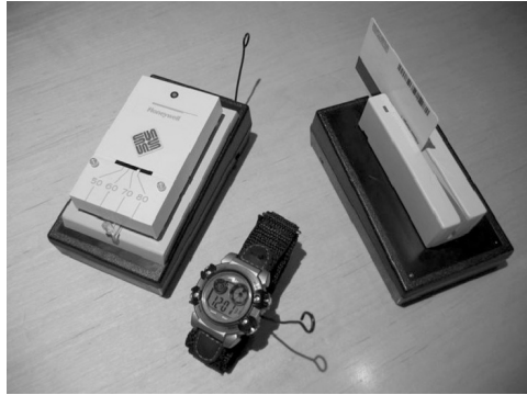
Fig. 6. ECC-enabled wireless devices built at Sun Labs: (a) thermostat, (b) health-monitoring watch (c) magnetic stripe reader.
