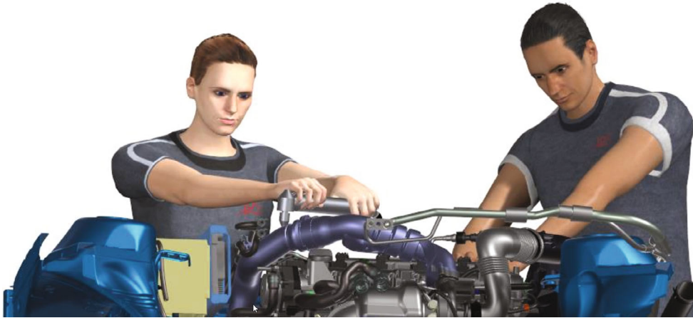
FIGURE 4 Simulation of the assembly of an engine of two workers in IPS IMMA.
